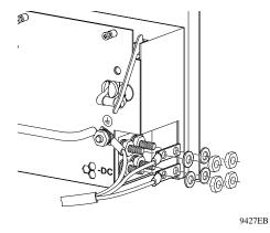
7. Disconnect the positive and negative voltage leads from the power supply terminals.
